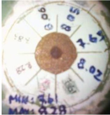
**Figure 3: A FBE sample after CD testing for 28 days at -1.5V and 65°C (holiday depth = 0.1 mm)**
