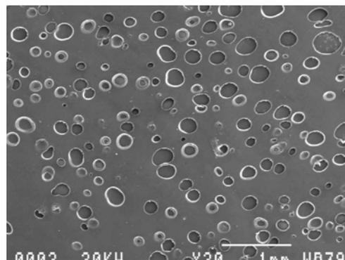
Fig. 9 SEM of Thermotite high performance polypropylene PP foam
