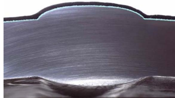
Fig. 3 Excellent coating coverage over a weld profile
