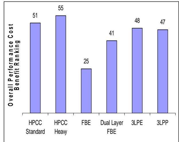
Fig. 7 Overall ranking of HPCC versus other coatings
