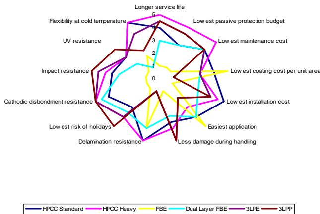
Fig. 6 A qualitative model for comparing pipe coatings
