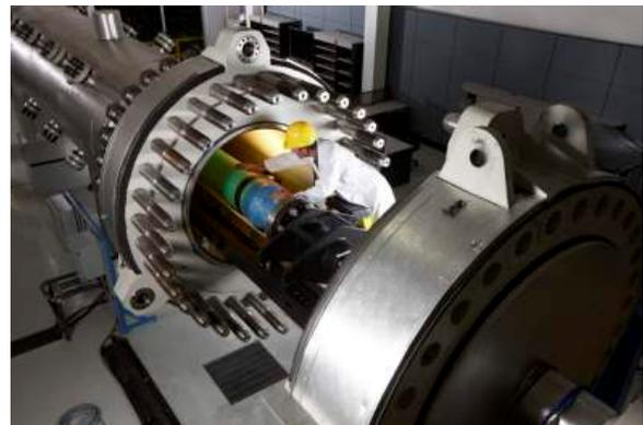
This pressure vessel simulates service conditions experienced by insulated subsea systems such as linepipe, field joints and, flexible pipe by applying pressure to water surrounding these systems while controlling the temperature inside the pipe. By measuring the heat flow, thermal conductivity and compressive creep of the insulating material, both the thermal efficiency and depth rating capabilities of the insulation can be confirmed. This data is used to verify design of the system.
