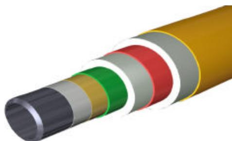
Figure 1. Thermal Insulation System for Single Flowline
