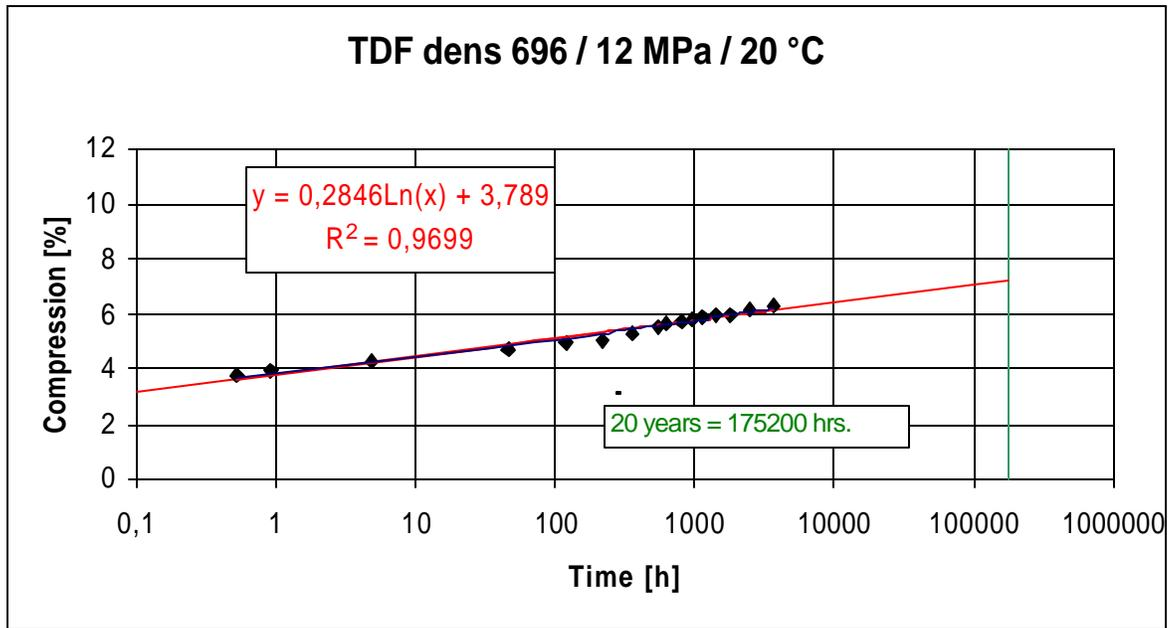
Figure 6. Creep Curve, 3712 hours for Novel PP foam
