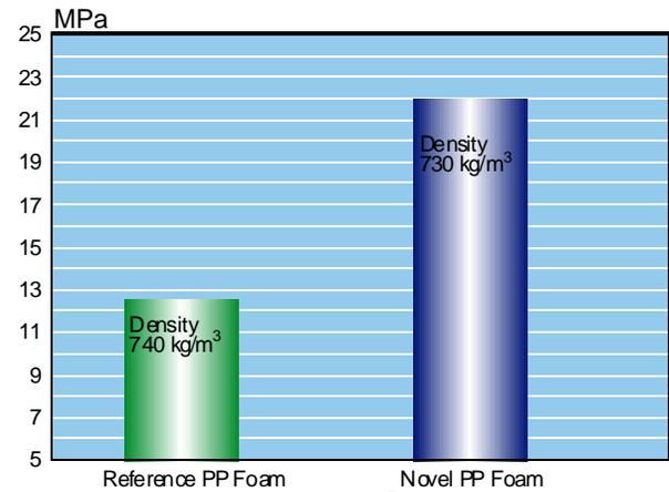
Figure 5. Compressive Strength @ 5% Strain Comparison
