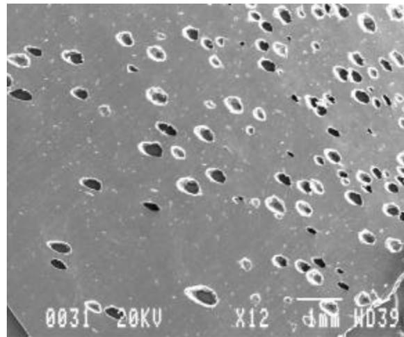
Figure 2a. SEM Photograph Reference PP Foam
