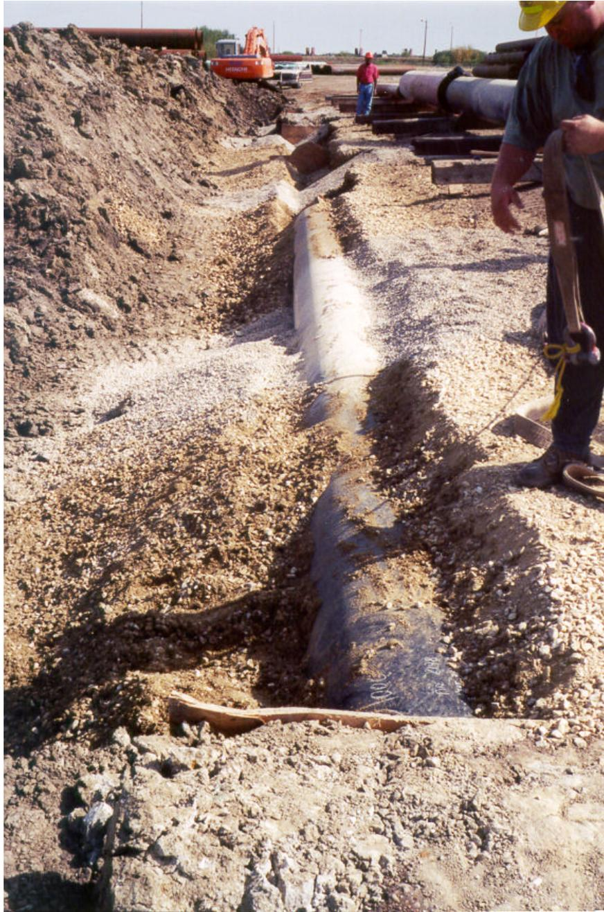
Figure 2. Completed test burial site for test pipes. The three gradations of crushed rock alternate in 4-m lengths along the full length of the trench.
