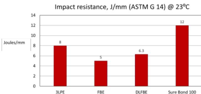
Figure 7 Impact resistance for various pipeline coating system at 23°C
