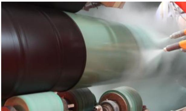
Figure 3 The reactive topcoat is extruded before FBE gelation to enable cross-linking reaction for bonding
