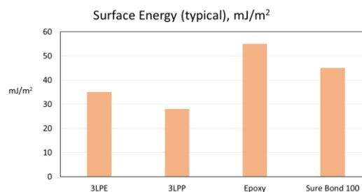
Figure 10 Surface energy values of different mainline coating systems
