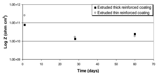
Figure 4 EIS results of 60 days at 95°C show the impedance of the new coating system close to that of a very good FBE
