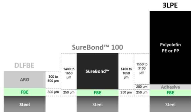
Figure 2 SureBond 100 configuration vs. DLFBE and 3LPE
