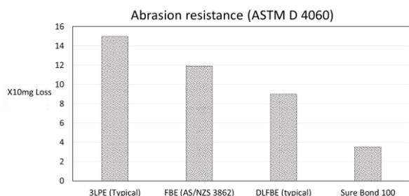
Figure 9 Abrasion resistance for various pipeline coating system (CS17, 1 kg load @ 1000 cycles)
