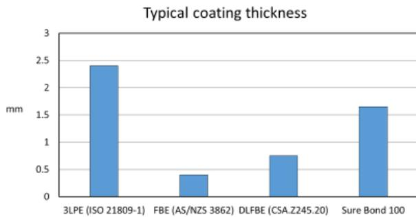
Figure 5 Comparison of various typical total thickness for various pipeline coating systems
