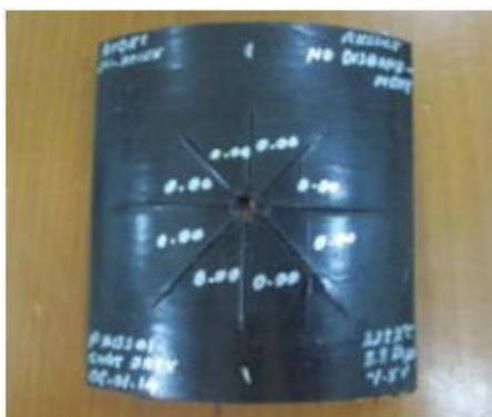
Figure 11 Zero cathodic disbondment was obtained after 48 hours at 65°C @ -1.5 volts
