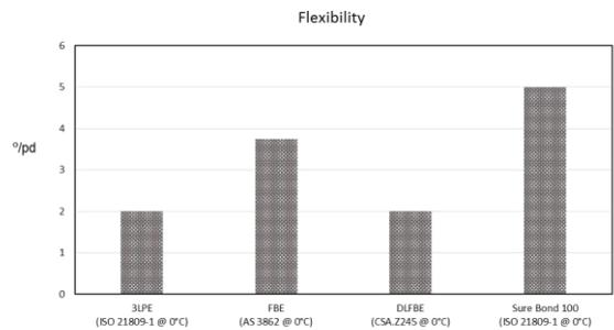
Figure 6 Average flexibility values for various pipeline coating systems at 0°C
