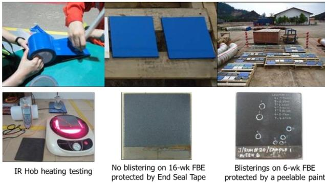
**Figure 4: End Seal Tape helped to eliminate FBE blistering during an IR Hob heating test**
