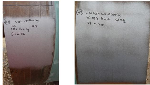
**Figure 5: Cutback preserved with End Seal Tape was easily blasted without affecting by residue after 1 and 2 week weathering**
