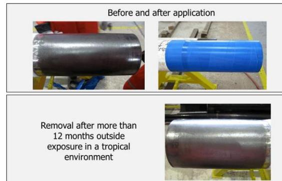
**Figure 3: A cutback area preserved with End Seal Tape after more than 12 month exposure in a tropical environment**
