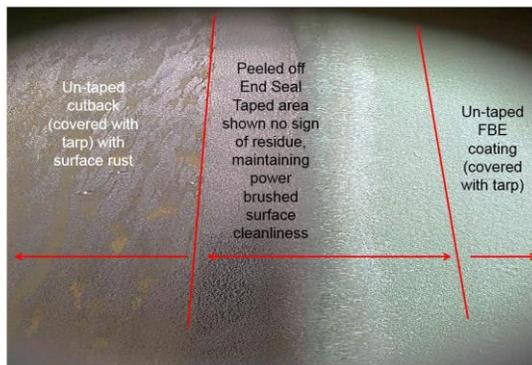
**Figure 2: End Seal Tape preserved the transition area of a FBE coated pipe over a month in a tropical environment**
