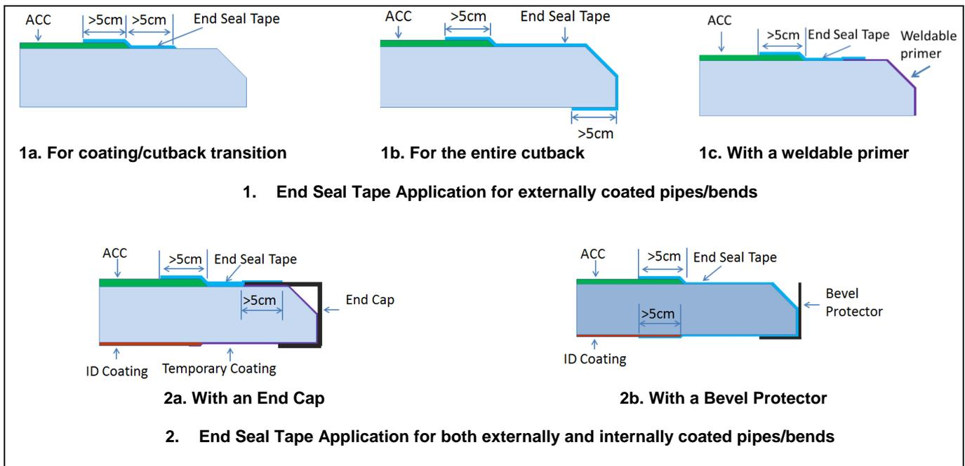
Figure 1: The use of End Seal Tape for different cutback options
