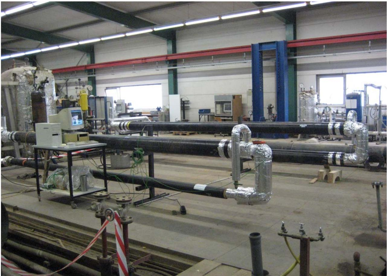
**FIGURE 4 - Insulated Pipe Accelerated Heat-Ageing (CCOT) Assembly**
