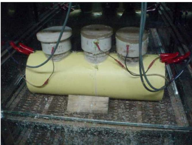
Figure 2 Cathodic disbondment resistance testing at 65°C
