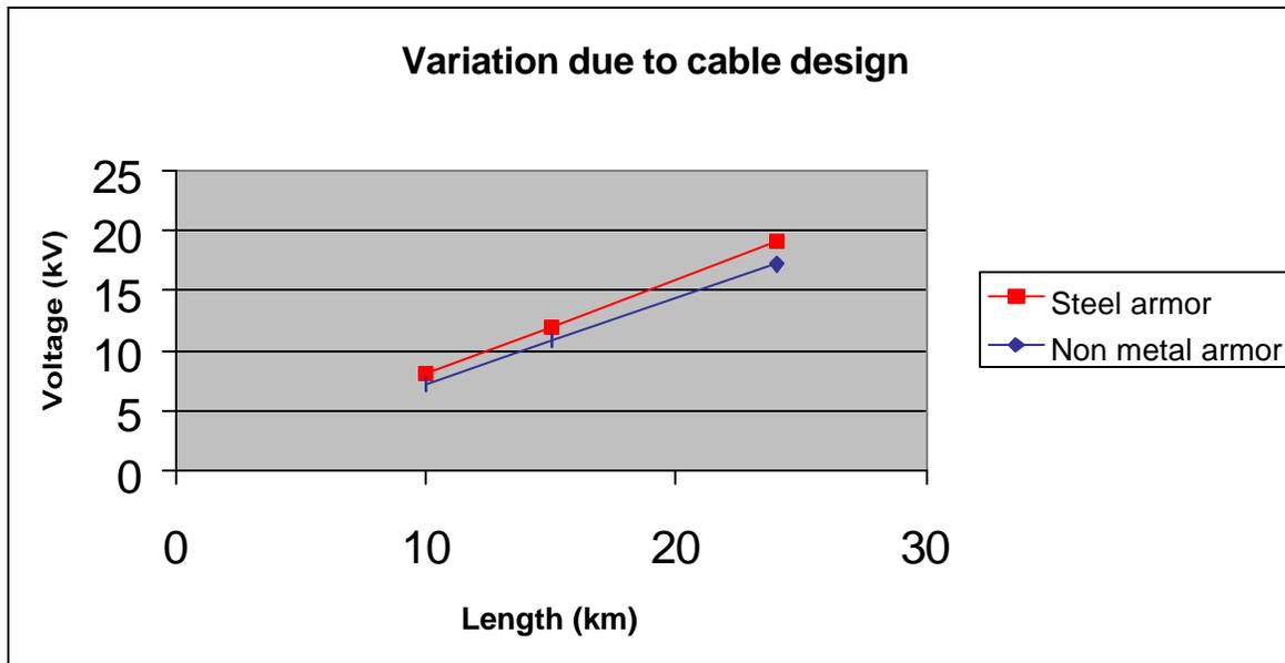
Figure 9-Voltage variation due to cable design, 100m spacing
