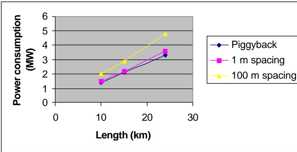
Figure 8-Power consumption as a function of length
