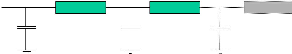
Figure 6-Equivalent p circuit
